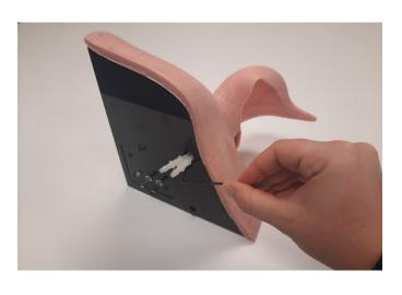
Close acrylic battery cover and tighten screws
